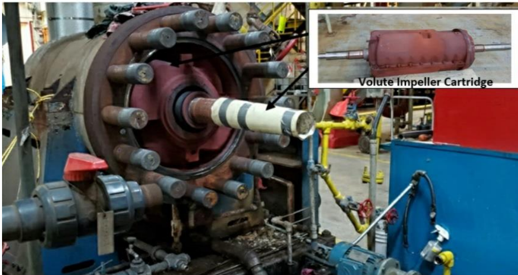
Figure 4: BF Pump Volute Impeller Cartridge During Disassembly
